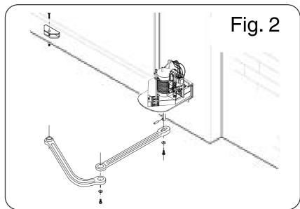
Insert the Ø10x14 pin and the straight arm into the shaft of the gearmotor and secure it with the M10x14 screw and 10x35 washer. Lubricate the pin of the straight arm. Join and secure the two arms with the M6x10 screw and 6x24 washer. Release the gearmotor and fix the curved arm to the bracket "A" with the M12x40 screw and the M12 nut, checking it is free moving. For application on the right-hand side see fig.2.
