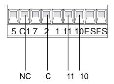
2. <u>For re-opening during closing.</u> Remove hard wire link between 2 & C1 and insert safety beam wires as shown.
