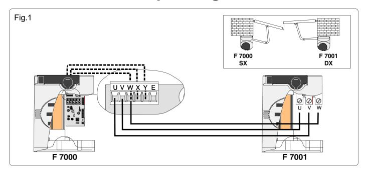
For gates with a delayed-closure left-hand gate, prepare the connection as shown in figure 1.
