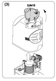
Open the lock cover cap (1). Push the key in and turn clockwise (2). Raise the cover, loosen the 3.9x13 screw and remove the cover from the gearmotor unit (3).
