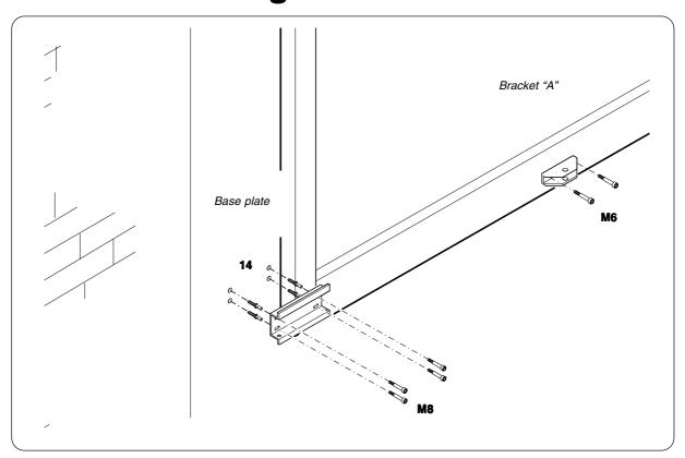
Using suitable anchor bolts or chemical resin for brick pier securely mount the motor plate to the brick pier. For wooden posts it is advised to fix the motor plate to the post. A threaded bar should be placed
