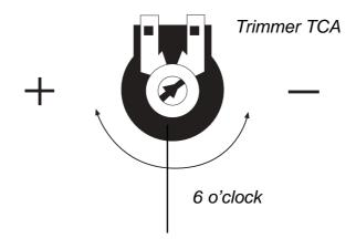
Fully anti-clockwise will automatically close the gates after approximately 10 seconds and fully clockwise will close the gates after approximately 80 seconds. A sensible setting is about halfway (i.e. 6 o'clock position) which will automatically close the gates after approximately 30 seconds.
