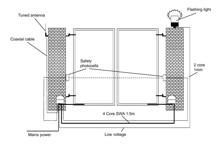
When installing low voltage cable around the gateway it is advised to put all low voltage cable in either ducting or alkathene piping. All cable jointing should be carried out above ground.
