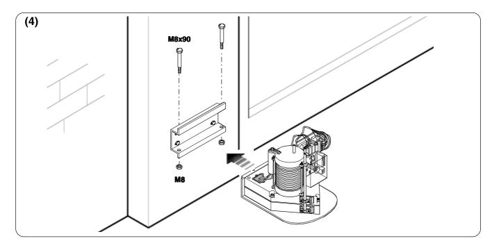
Insert the gearmotor in the base plate, align with the 4 holes and secure it with the two M8x90 bolts and nuts provided.
