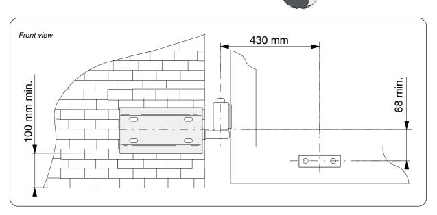
Use M8 screws and Ø14 screw anchors to mount the base plate on the pillar. Be sure to respect the 100mm minimum distance from the pavement. Attach bracket "A" to the gate wing (use M6 screws or welds). Be sure to respect the offsets of 430mm and 68mm.
